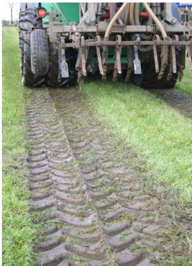
It is commonly known that both tire pressure and wheel load contribute significantly to soil compaction. Innovative measures are needed to ensure improved distribution of the weight impact on the soil. Photo: Janne Hansen
