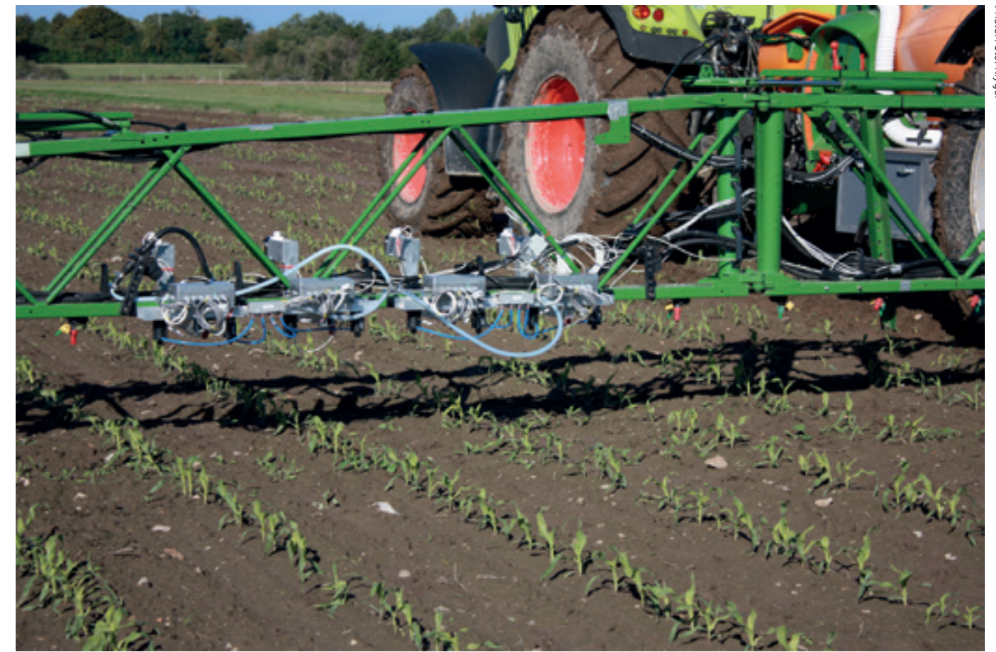
Researchers from Aarhus University are involved in the development of integrated pest management methods, including an intelligent spray boom that can reduce pesticide consumption by up to 60 per cent.
