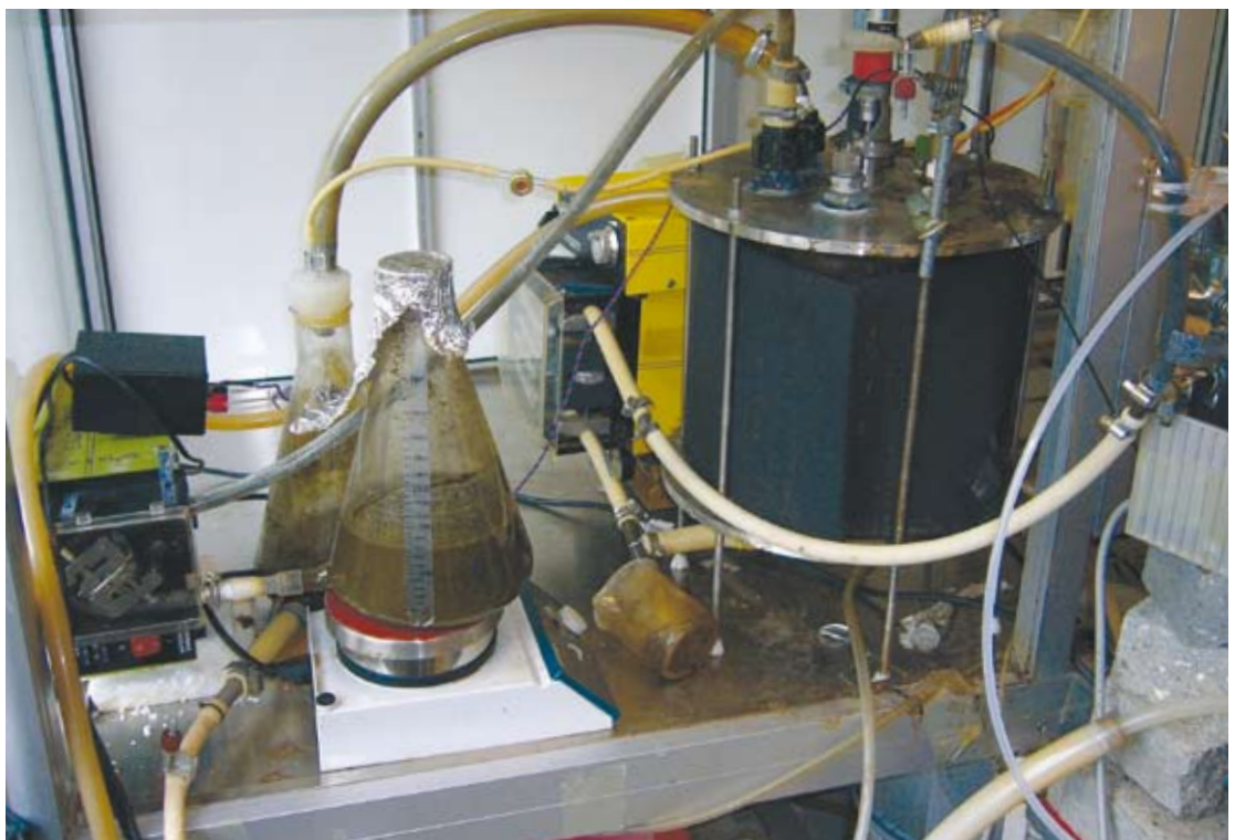
Figure 18. Laboratory setup to measurement of biogas.
